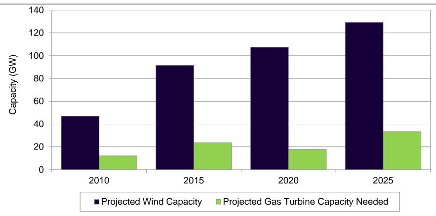
Note: Assumes the required gas turbine capacity for firming wind generation is 25.8 percent of the installed wind capacity and the average annual utilization of gas turbines for firming purposes is 15.6 percent. Source: ICF International.
