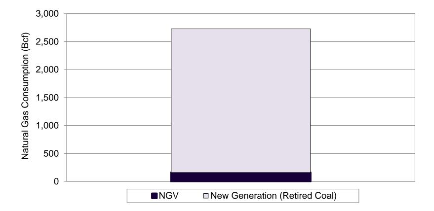
Note: Assumes 160 Bcf of NGV natural gas use. Also assumes retirement of 45 GW of coal-fired capacity, replaced with new natural gas generation with an 85 percent capacity factor and a 7,600 Btu/kWh heat rate.
